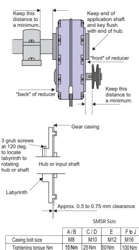
The Vee - belt dtive can be located at any convenient position but if the torque arm is to be used for belt tension the angle shown below should be approx. 90 deg. The Vee - belt drive can be located to the left if required.
